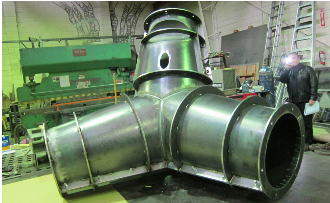
Steel form for casting concrete pods
